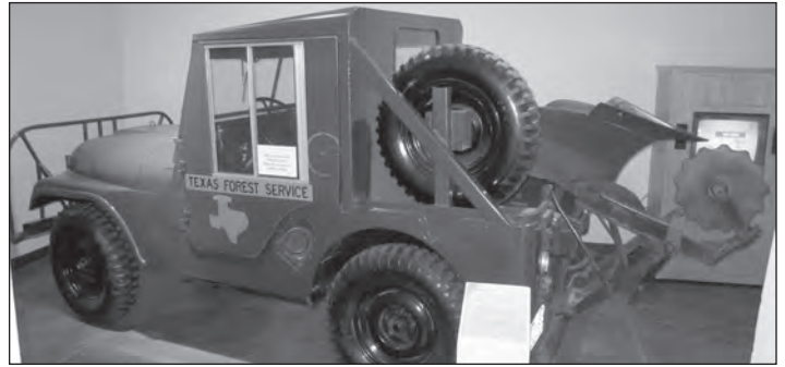
A Texas Forest Service Jeep, which is designed to pull a fire plow.
